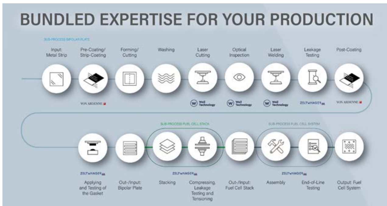
GERMAN FUEL CELL COOPERATION: Process chain for the production of fuel cell systems (© German Fuel Cell Cooperation)
