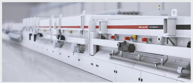
VON ARDENNE GIGA|nova DCX – PVD coating tool for high-volume manufacturing with an annual capacity of up to 1.3 GW (© VON ARDENNE Corporate Archive)
